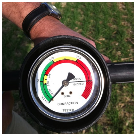
Figure 2. A closeup of a penetrometer face, showing the amount/thresholds of resistance.
